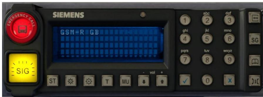
Beginning in 2013 and completed by 2016, Global System for Mobile Communication - Railway, more commonly known as GSM-R, replaced the existing National Radio Network (NRN) & Cab Secure Radio (CSR) systems. A simple version of this communication system and its accompanying unit has been simulated.
