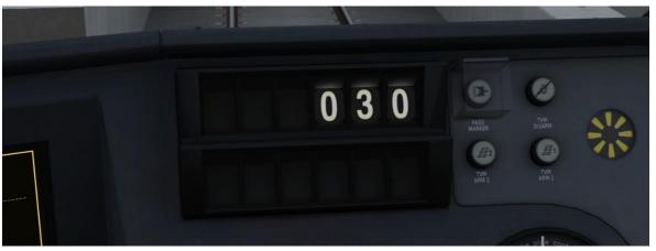
TVM-430 is the signalling system used on the high-speed line section of the London – Faversham route and is simulated in this pack. When on this line, make sure to select 'BR CTRL' on the 'system selector switch'. Please consult the manual for that route on how this signalling works.
